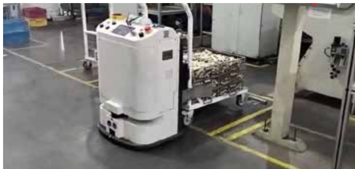
FORKLIFT AMR - SLAM NAVIGATION
